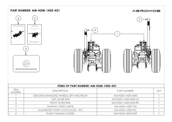
APPROVED USE: The HARDMOB 145D equipment has the function of suspending the aircraft from the ground and enabling the movement of the landed helicopter. The HARDMOB 145D is approved for use on Airbus H145D2 and H145D3 model helicopters in all versions, including Mercedez versions that have fairings on the
